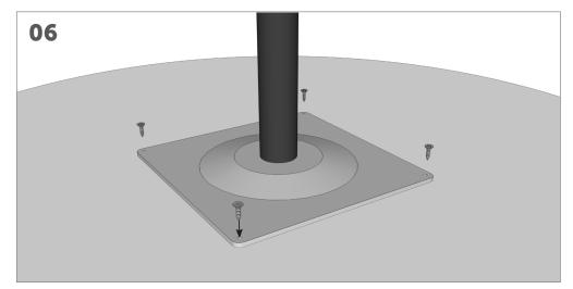
Fully tighten the last 4 self tapping screws into the work surface.
