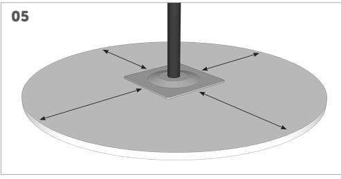
With the frame assembled, place it upside down onto the work surface, and measure the top from all sides to make sure it's centered.
