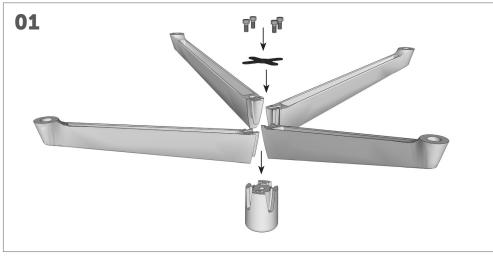
Slide the 4 large feet into the cross collar. Place the cross gasket on top of the feet and collar, and tighten 4xM5 screws into the cross collar.
