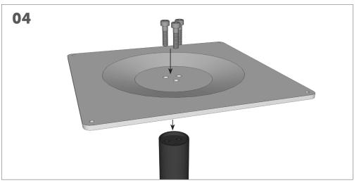
Locate the steel plate on top of the feet tube, and line up the 3 holes. Fully tighten the 3 screws into the tube.
